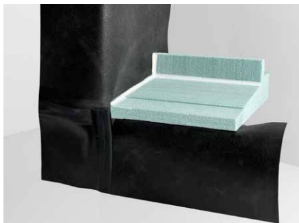
Wedge with junction to rear ventilated facade (EPDM outer corner)
